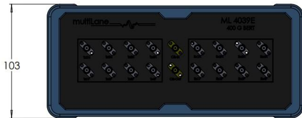
Figure 3: ML4039E front view with dimensions
